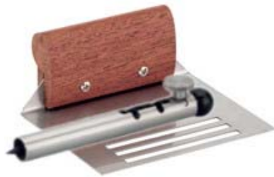
Cross cut device to test the surface strength
