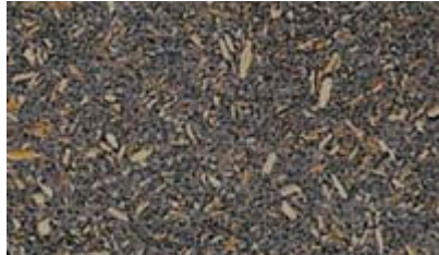
Structure of cement fibre board
